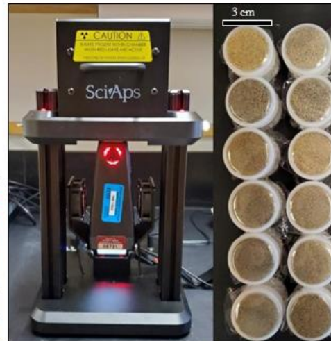
Figure 1. Generalized pXRF screening considerations for detecting critical commodities contained within offshore sand resources. Ex-situ sample pucks include packed sediment with a 4-micron thick prolene protective sheet.
